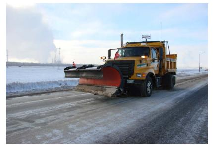
*Ice and Traction Control* is the application of a sand/chemical mixture or pure chemical to the road surface in order to increase the traction of vehicle tires in winter conditions.
