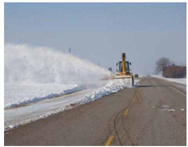
Snow removal operations involve the removal of snow from the road rightof-way using trucks, industrial snow blowers, and front-end loaders. These operations will commence once other snowplowing operations have been completed. Snow is then transported to approved snow dumpsites, where the snow is stored until the spring melt. Snow removal ensures that there is snow storage capacity for future snow clearing operations and improves driver visibility within the right-of-way.
